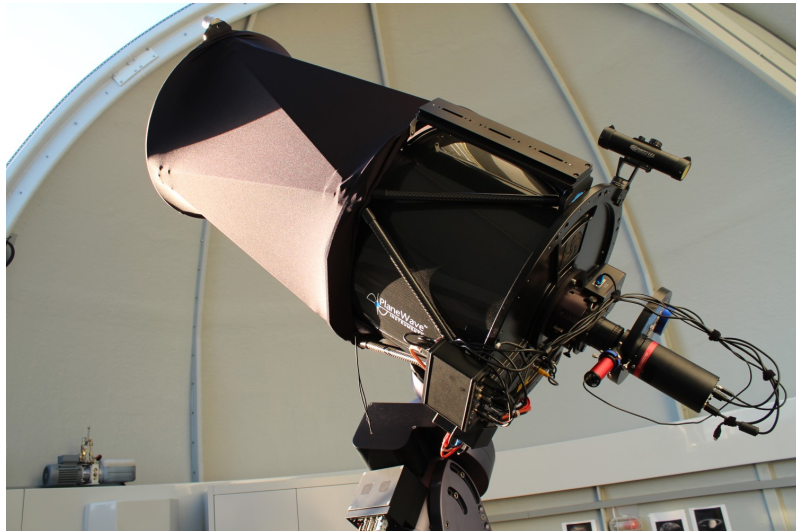
(b) The inside of the dome with the CDK20 on top of the 10Micron mount in the center. (The image has been taken from the OST Wiki page)
