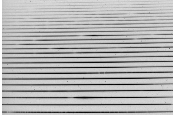
Figure 5.6: An echellogram, like it forms on a camera sensor (brightness inverted). This is a spectrum of V1405 Cas. It is a stack of 3 images, each exposed for 2000 s, taken on the 10.05.2021 at the OST as part of our observations.
