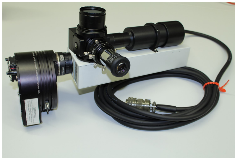
Figure 5.3: An image of BACHES - The high resolution echelle spectrometer, utilized to perform this observation, with the SBIG St8 camera attached to it. This image has been taken from the OST Wiki page.
