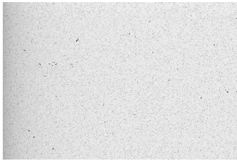
(a) This is an arbitrary (brightness inverted) dark frame (1000 s exposure time at -20^{\circ}\text{C} camera chip temperature).
